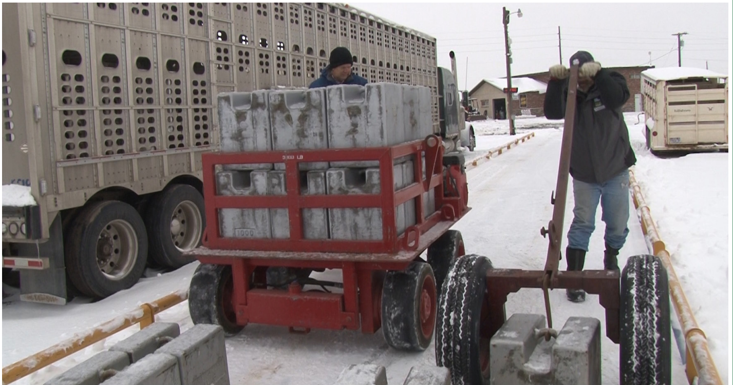
Large scale scales are usually not mobile and must be inspected on site. The photo above shows the older, more labor intensive method of inspecting and calibrating large truck scales. In recent years the department has been adding new trucks with more automated equipment, which is safer, quicker and more efficient for inspectors.
